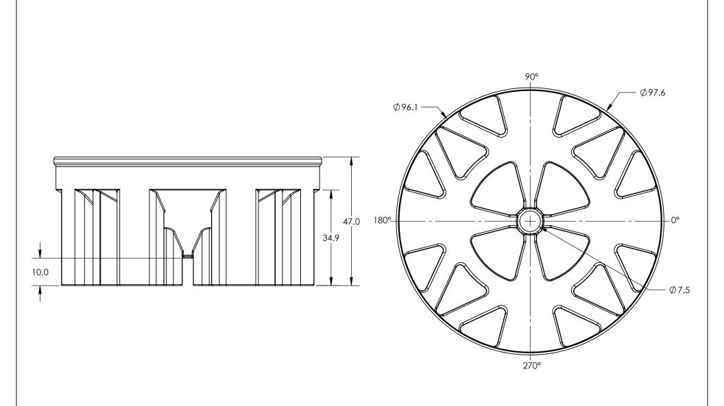
\*ALL EXTERNAL PIPING MUST BE INDEPENDENTLY SUPPORTED. \*ONLY BASE FITTINGS TO BE LEFT INSTALLED AT TIME OF SHIPMENT PER SII PROCEDURE. ALL DIMENSIONS ARE IN INCHES, NOMINAL, & SUBJECT TO CHANGE WITHOUT NOTICE. ALL DIMENSIONS ON ROTATIONAL MOLDED PARTS ARE SUBJECT TO A  $\pm$  3% TOLERANCE.
